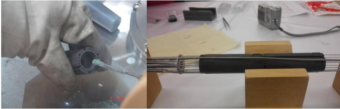
*Filling of crucible with sample salt at JRC Karlsruhe (left) and assembly of sample holder at NRG (right)*
